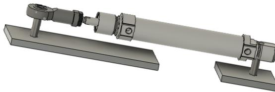
Figure 2.12: Illustration of how two spacers would be connected to the pneumatic cylinder. The two rectangular blocks that the cylinder is connected to represent two moving parts of the fixture.
