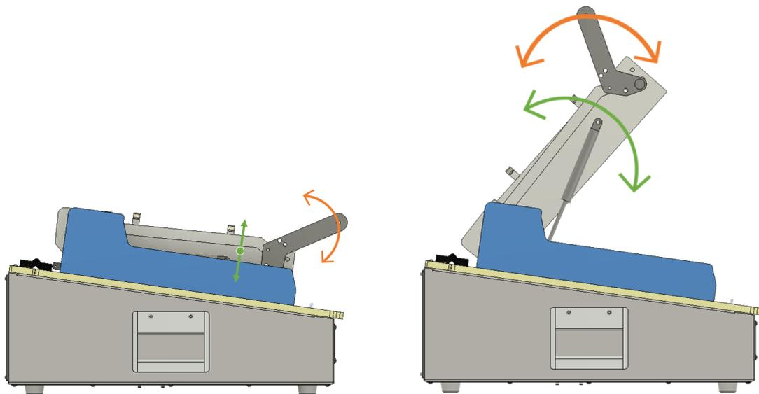
(a) This motion will be called locking or unlocking depending on the direction of the lid.
