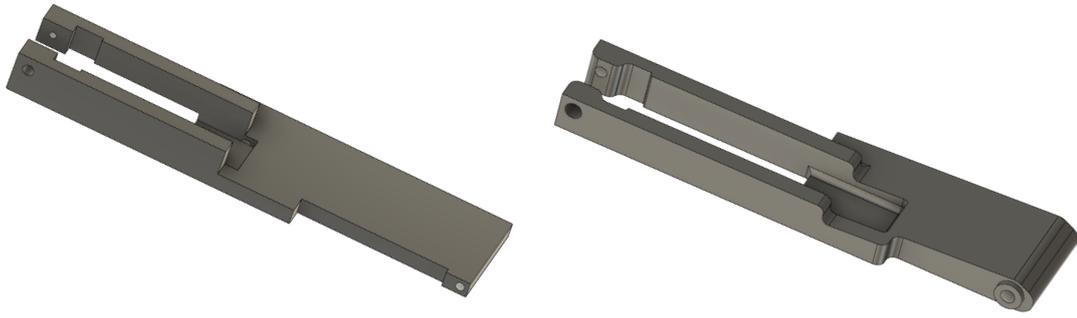
(a) Side plate designed for CNC manufacturing.
