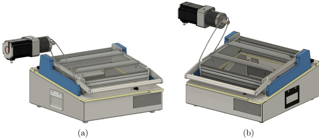
Figure 2.3: A rough illustration of how a chain could be fastened to a servo to automatically open and close the FCT-fixture.
