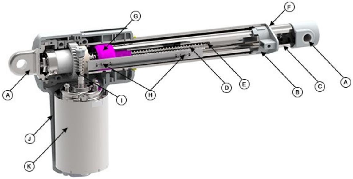
Figure A.1: Se through image of an electric linear actuator. [19]
