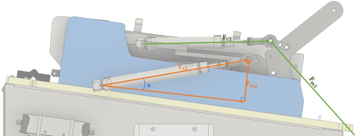
Figure 2.9: Illustration and notation for force calculations.  $F_{m1}$  is perpendicular to the handle.
