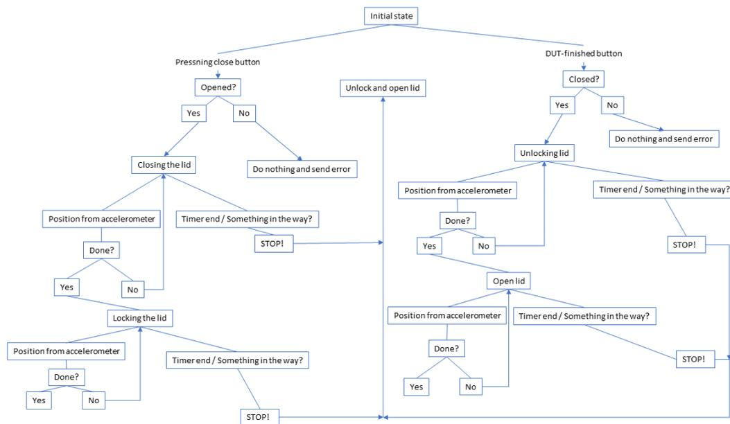
Figure 2.7: Flowchart over how the code should be generally implemented.
