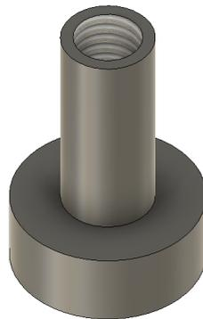
Figure 2.14: The spacer used to fasten the lower part of the lower cylinder to the fixture.
