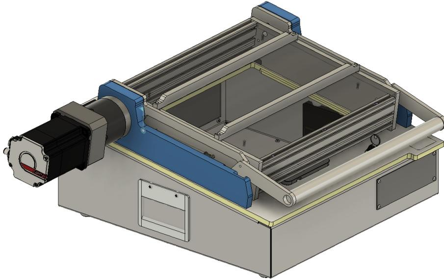
Figure 2.1: Illustration of how a servo could be placed to open and close the FCT-fixture.
